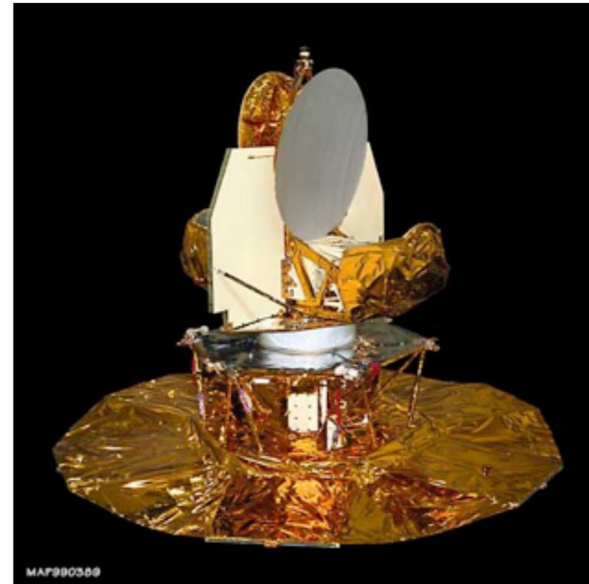
Note the same dual receivers as COBE. This design, plus the very stable conditions at the L2, minimizes the “ $1/f$  noise” in amplifiers and receivers.
