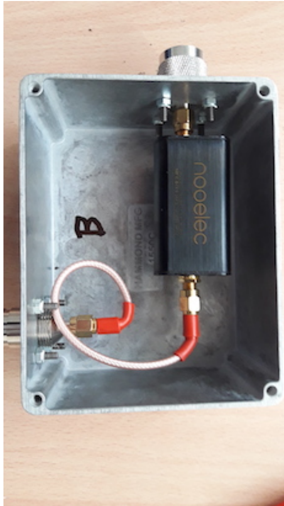
Fig. 9.7.2: View inside the aluminium box hosting the HEMT and band pass. This device amplifies the signal and limits it to the HI 21-cm line at 1420.4 MHz. Because of mechanical stability the aluminium box is equipped with N-type connectors. Within the box the SMA type connectors are used. This device need a DC voltage. It is provided by the bias-tee element and the connected high frequency cable.
