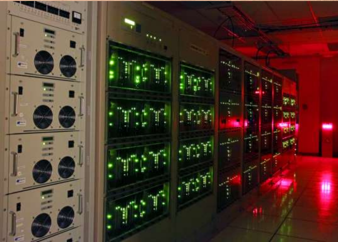
One of the four quadrants of the main array correlator
